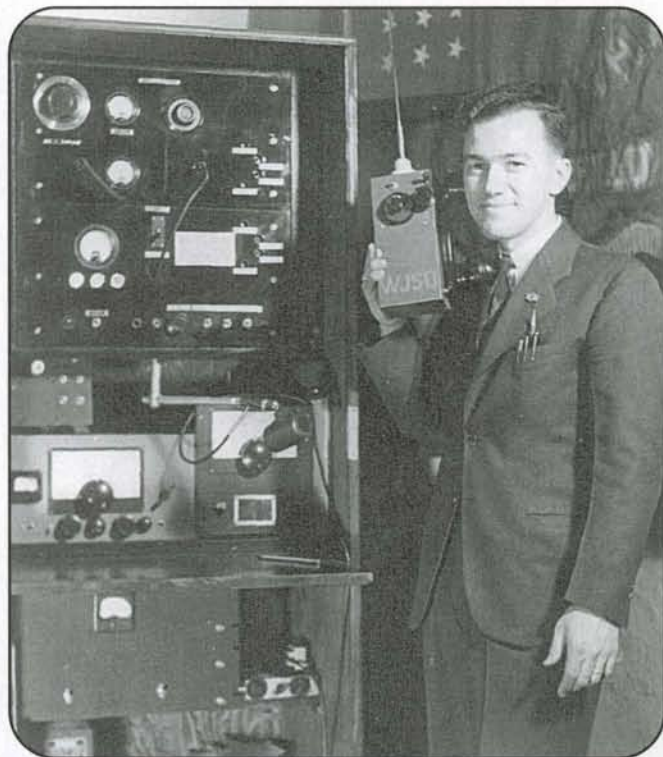
Photo 4. In 1942 Jim designed and built the War Emergency Radio Station (W.E.R.S.) used by the town of South Plainfield and assigned the special call sign WJSQ by the FCC. This is the station.
