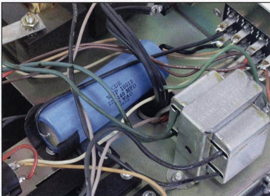
Photo 9. This photo shows the terminals in the upper right. The blue starting capacitor is also shown.
