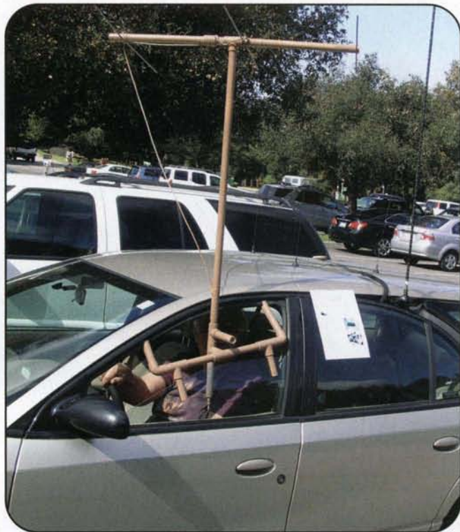
Bob Thornburg, WB6JPI, brought a prototype of his simple 3-element T-hunting Yagi and mobile mount to a recent ARDF session to get comments and suggestions.
