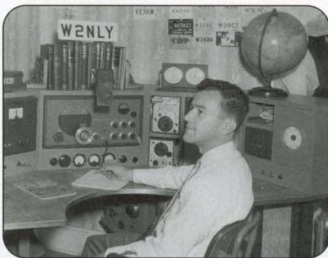
Photo 10. Jim at the operating position of his Oak Tree, NJ QTH. The station consisted of a 2-meter converter and a Panadaptor that he built himself, as well as an SX-42 receiver. The unit on the far left is a narrow-band IF device that he used for experiments with Walt Bain, W4LTU.
