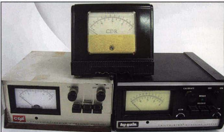
Photo 1. Examples of three rotor controllers. The top one sports a single lever-operated switch and a large meter. The bottom two show the later additions of the direction control and brake switches (lower right in both controllers), as well as the calibration and on/off switches (upper right on both controllers). (Photos by the author)
