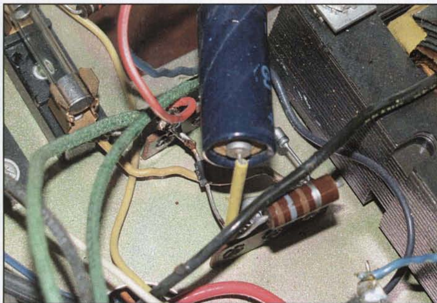
Photo 2. An example of point-to-point and point-to terminal wiring. The zener diode is wired between two terminal strips in the center of the photo. The location of the 3-amp fuse is in the upper left corner of the photo.
