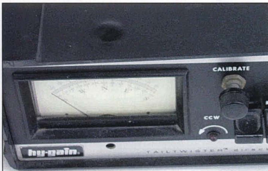
Photos 6, 7, & 8. These photos illustrate the effect of the hot bulb on the plastic cabinet. Note the bubbling of the cabinet just above the meter in photo 6 (left) and in front of the meter in photo 7 (bottom left). This effect is why it is necessary to ensure that the duct tape shown in photo 8 is securely in place. Both photos 7 and 8 (bottom right) also show the starting capacitor, which is blue.
