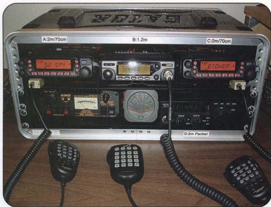
Photo 5. This VHF/UHF amateur radio station is an excellent example of how to organize a portable EmComm station. (Photo courtesy of NC6T)
