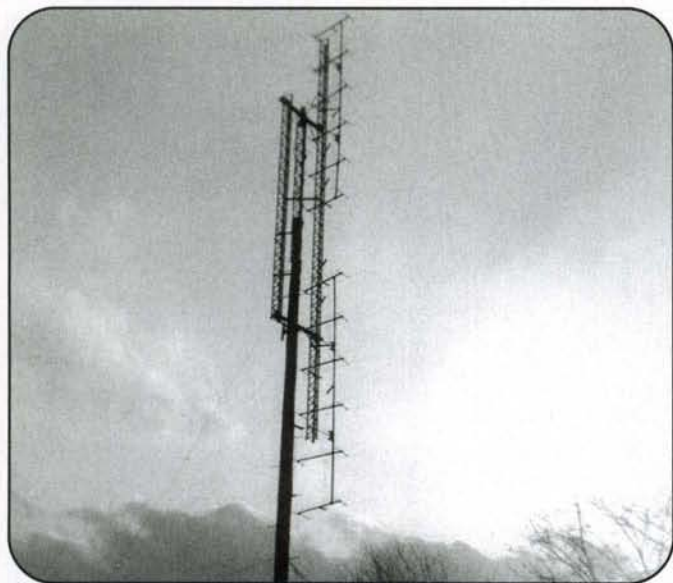
Photo 13. In 1954, Tommy Thomas, W2UK, and Paul Wilson, W4HHK, in Tennessee, were credited with the first-ever meteor-scatter QSO on 2 meters. In an effort to pick up Tennessee as a new state, Jim created the new 48-element antenna shown here.
