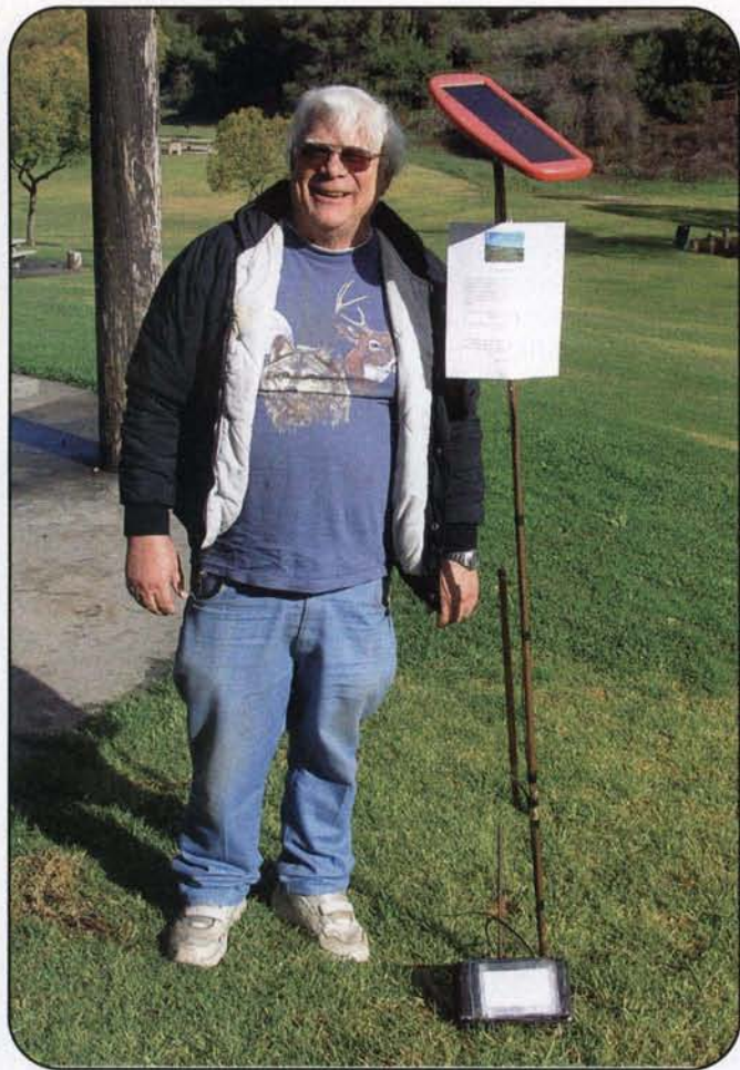
WB6JPI proudly stands beside GeoTran. Its solar panel is mounted atop a copper-pipe J antenna for 2 meters.
